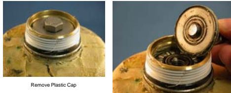
Unscrew Bolt, Remove Thrust Washer
